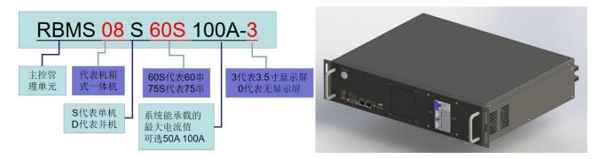
For example: RBMS08-S60S-50A-0, which means the case-type all-in-one is a single machine, suitable for 60S lithium iron phosphate batteries, supports a maximum current of 50A, no LCD display.
