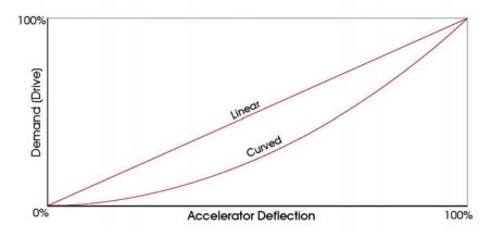
This sets the type of response for the Accelerator Input (pins 8 or 9 on Connector A). There are two options for AC Traction control, Linear and Curved.
