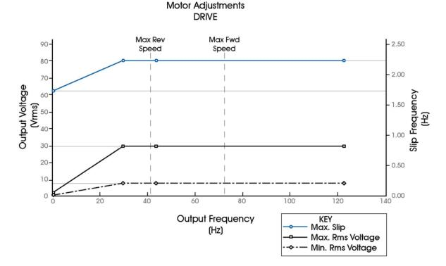
The 'basic' motor set-up for drive is now defined. Depending on the feedback from the speed encoder and the torque demand from the accelerator, the controller will vary the voltage between the minimum and maximum values shown on the graph. The slip will vary between 0Hz and the maximum setting for the given speed.
